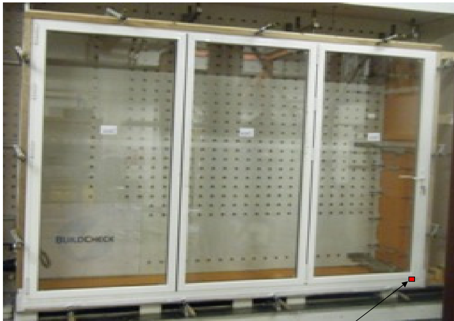
Leakage 1 min 15 sec @ 200Pa
